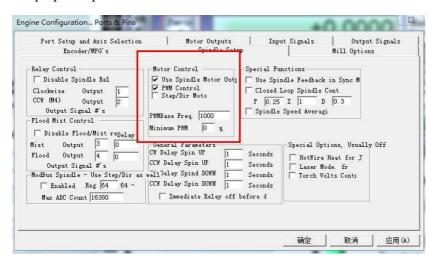
Enable spindle output. as shown below:
