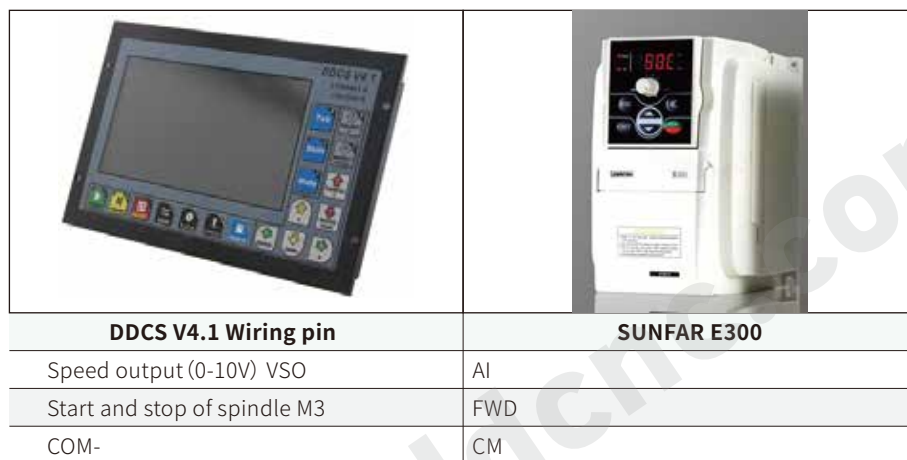
Figure 2-9 DDCS and VFD wiring
